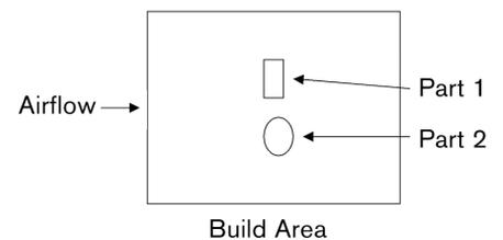
Figure 2: Build area configuration Position parts as close to the center as possible.
