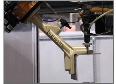
Figure 4: FDM EOAT gripper used in a waterjet operation.
