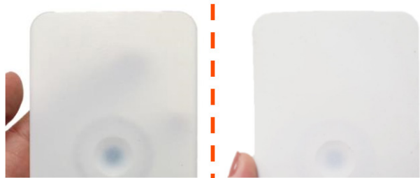
Figure 2: Material opacity—partially translucent with Vero materials (left); fully opaque with VeroUltra opaque materials (right)
