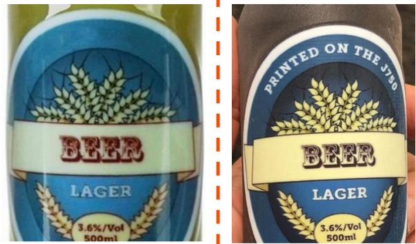
Figure 1: Thin label with text printed in full color on J55—blurred with Vero materials (left); sharp and realistic with VeroUltra opaque materials (right)
